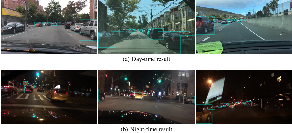
Figure 2: Visualization of traffic object detection results of Mobip. (a) Results in day conditions and (b) Results in night conditions
